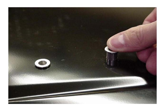
10.Locate protective gaskets on roof panel; install roof rack assembly on gaskets. Install one ½"-20 screw in each side rail support. Make sure gasket is aligned with supports. Install second ½"-20 screw in supports, then tighten rearmost screws first. Repeat for remaining screws. Torque screws to 50 inch-pounds. Please see the sketch below for the proper tightening sequence.
