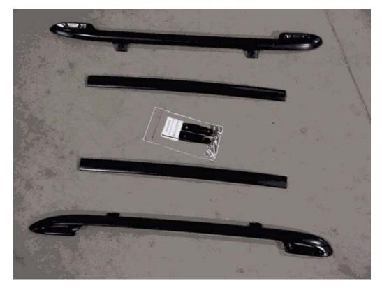
2. Attach cross bars to side rail assemblies with 5mm stainless steel screws. The resultant assembly should be as shown below.
